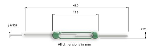
This form A reed switch is built with a 2.25 mm diameter glass having a higher wall thickness for better glass to metal seals, and is a good solution for general purpose, high volume applications with a little shock and vibration, such as toys. The centre contact also makes it suitable for coil applications. The three differential ranges available cover a wide range of release specific applications. A specially plated contact for 230 VAC line voltage switching is also available.
